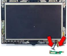
15. Connect the 2 cables to the power switch board and place it into the rear cover.
