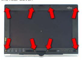
17. Press the front cover into place and secure it with 8 screws.
