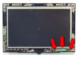
7. Extract 2 screws from the power switch board and turn it over.
