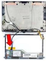
10. Turn the LCD over remove the tape from its cable and disconnect it.
