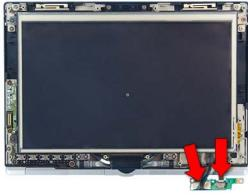
8. Disconnect the 2 cables from the board and lift it out.
