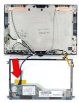
13. Connect the LCD cable, tape it down and place the LCD into the rear cover.
