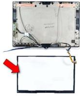
12. Replace the defective part and place the LCD onto the digitizer. Be sure there is no dust between them.
