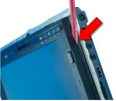
4. Using the plastic pry tool pry around the perimeter of the display to release the front cover from the rear.
